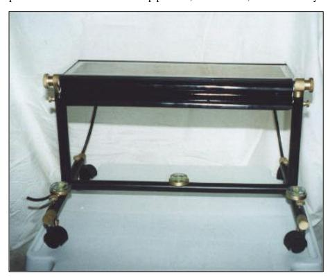
checked atmosphere and the four wheels that allow the structure to move in any direction. For the lifesize realization, because of the weight we recommend the movement automation by means of a directional remote control that through a joystick will allow the displacements (like radiocontrolled miniatures). This configuration encumbrance is 5.3 m length and 3.6 m width. The height is 3.1 m ca.
