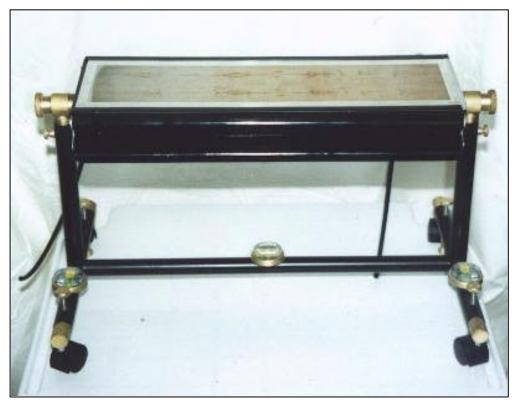
In the third image there is a side-view of the structure that should contain the Shroud in which one can note the faucets on the back that allow the entry and the exit of the gas for the checked atmosphere inside the Shroud container. The pipes that were applied are purely indicative,
