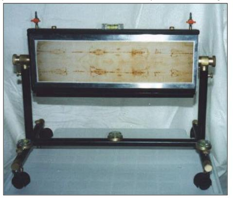
This seventh image shows the Shroud container with the upper cover removed. You can note how the Shroud, inside the container, is less visible than the photograph outside because of the protection glasses. The use of photochromatic glasses should be also considered. They are sensitive to the light and will allow for good visibility of the Shroud, but won't let the Shroud itself suffer
