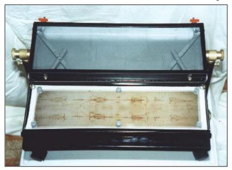
operations the control of inside system the atmosphere is temporarily disconnected with closing of the faucets. The drawer could be easily removed, for possible new examinations, or drawings by means of the anchorages at the two pantograph arms that are visible immediately above the Shroud. Obviously a table on which to place container must also provided.
